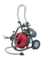
**Electric cable feed and rewind**. Steel-core cable: very flexible, very strong. Cable feed guide adjustment. Clutch release for automatic cable feed. Electric cable winder. Removable metal drum. Opens for cleaning and lubrification. Portable folding trolley.
