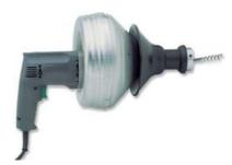
Manual cable feed and rewind Steel-core cable: very flexible, very strong. Variable speed control. Cable feed guide adjustment knob. Cable locking handle. Lightweight alloy drum. Supplied with Ø. 8 mm cable. 7,5 m long with boring gimlet.
