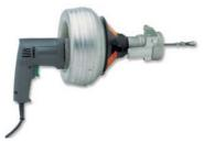
**Electric cable feed and rewind.** Steel-core cable: very flexible and very strong. Variable speed control. Cable feed guide adjustment knob. Cable locking handle. Manual clutch release for automatic cable feed. Lightweight alloy drum.
